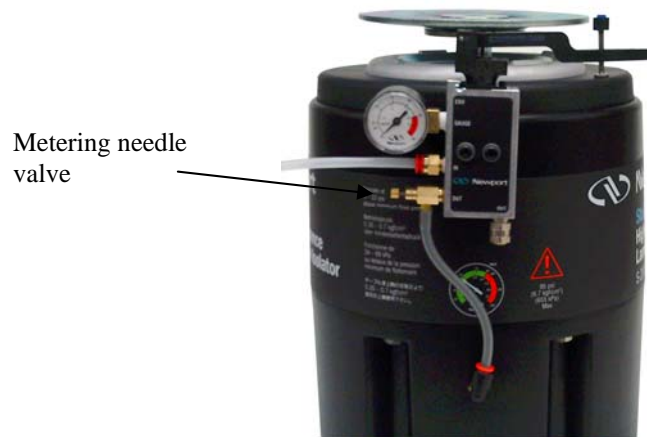
Figure 9 — Detail of Valve Connections, Single Isolator
