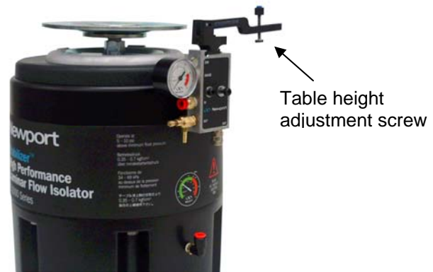
Figure 6 — Valves attaching to isolator
